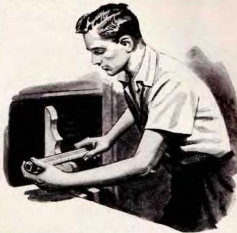
When sanding the edge of an inside curve or circle, the work goes much faster and easier if the sandpaper is wrapped around a piece of pipe about 6 in. long. The diameter of the pipe will depend on the radius of the curve to be sanded. Using the pipe also helps to keep the sandpaper square with the work.
